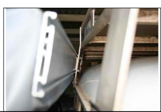
You can fix the awning on a vertical surface by simply drilling 4 holes with the desired distance and use the sliding bolts to fix the awning directly to your car/basket.
