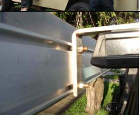
Fix the awning to the mounting brackets with M6 bolts.
