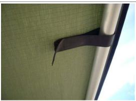
Fix the awning material to the frame with the Velcro fasteners.
