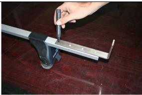
Make sure all L-brackets are aligned and have the desired distance to your car before you mark the drilling holes on your rack.
