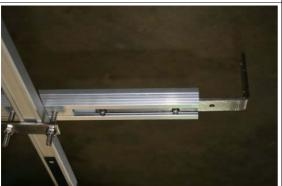
Slide them to the desired position and fix the bracket with fitting nuts to the mounting rails.
