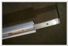
Use the groove of the roof tent mounting rail to slide in the mounting brackets with the M6 bolts in place.
