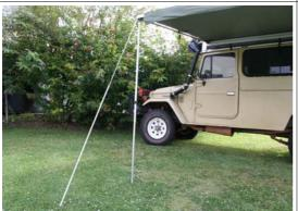
Use ropes and pegs to fix the awning securely to the ground.
