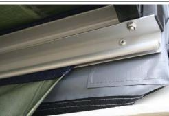
Slide the tent walls into the sail track at the bottom of the awning mounting plate.
