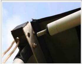
Feed them into the designated opening on the outer frame and extend them to tension the awning material.
