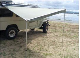
During rain and unsupervised periods, always lower one leg to allow rainwater to run off the awning and avoid pooling.
