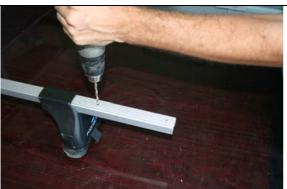
Drill at least 2 holes for each bracket. We highly recommend to take the racks off your car for this procedure.
