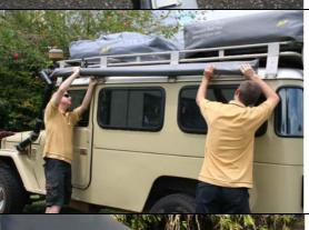
Make sure the awning is the right way around. Use two persons to lift it in place and fix the bolts at the back of the mounting plate to the mounting brackets.
