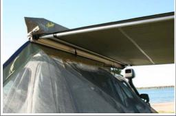
Slide the mosquito net into the sail track at the bottom of the awning mounting plate.
