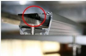
The head of the bolt will be held in place from the roof tent mounting rail.
