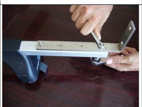
Fix the brackets to your rack by using M6 bolts at the necessary length and tensile strength.
