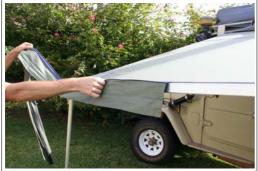
Feed the outer zip flap into the sail track of the awning. This part needs to be fixed for the very first assembly only and can remain on the awning.
