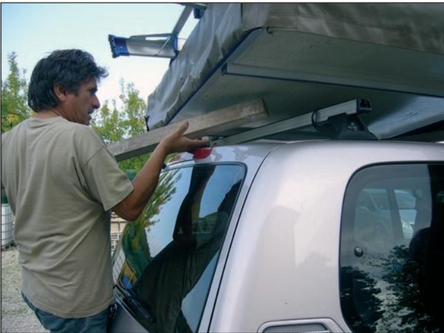
5. Attach the roof top tent to your roof bars in two places. Use 2 bolts and 2 slide plates with the base to hold the bar.
