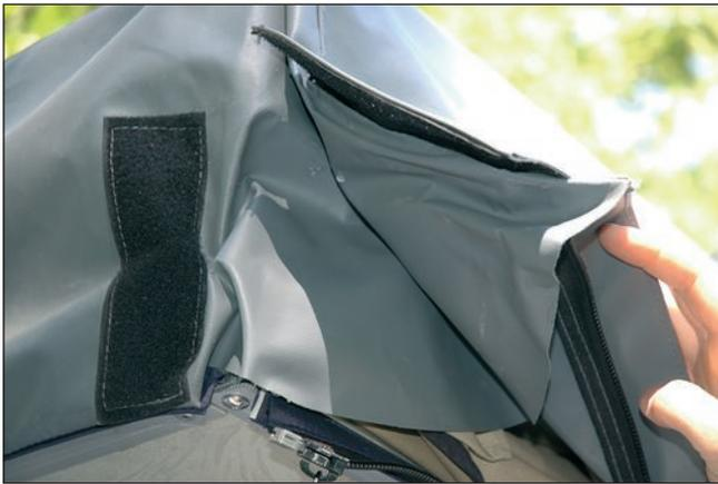
3. Remove the PVC travel cover from the tent by unzipping around three edges and slide the remaining edge from the rope track. Keep the PVC cover on until the set up is finished.
