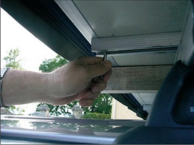
4. Remove the lintel and put it near the other roof bar.
