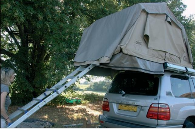
**Special note :** Although the tent structure is able to support itself in an emergency, the ladder is required for support at all times for normal use.
