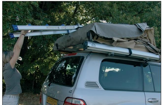
8. Pull down on the ladder, which will now lift the top half of the tent. Make sure that the two halves of the tent engage properly and the tent floor is flat.
