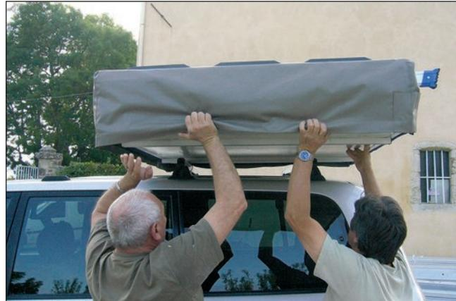
2. Insert a lintel between the tent and the roof bars in order to fix the bolts easily
