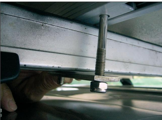
6. Prior to tightening all the nuts, ensure that your roof top tent is centered (side to side) on the roof of your vehicle, and the mounting points (as far as possible) are symmetrically positioned near each corner of the tent.
