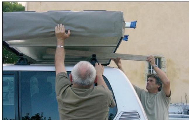
3. Place 1x8 mm bolt into the slide plate. Slide the plate and bolt into the mounting extrusion.
