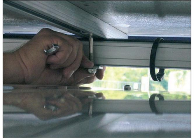
9. Remove the lintel definitively and attach the roof top tent to the second bar, as for the first one.
